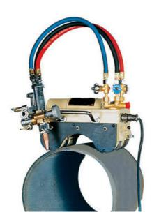
Model HY-2399 is a supper pipe cutter with a meganetic system which can attach the machine without binding to the pipe firmly for steady cutting which avoides the machine drops off accienditly, but still It's recommend that the adjustable guide belt be used for quicker set-up and improved cutting accuracy, Esp. for large size pipe cutting, Bestls are available for 10" above, Pipe sizes up to 42" ca be accommodated.
